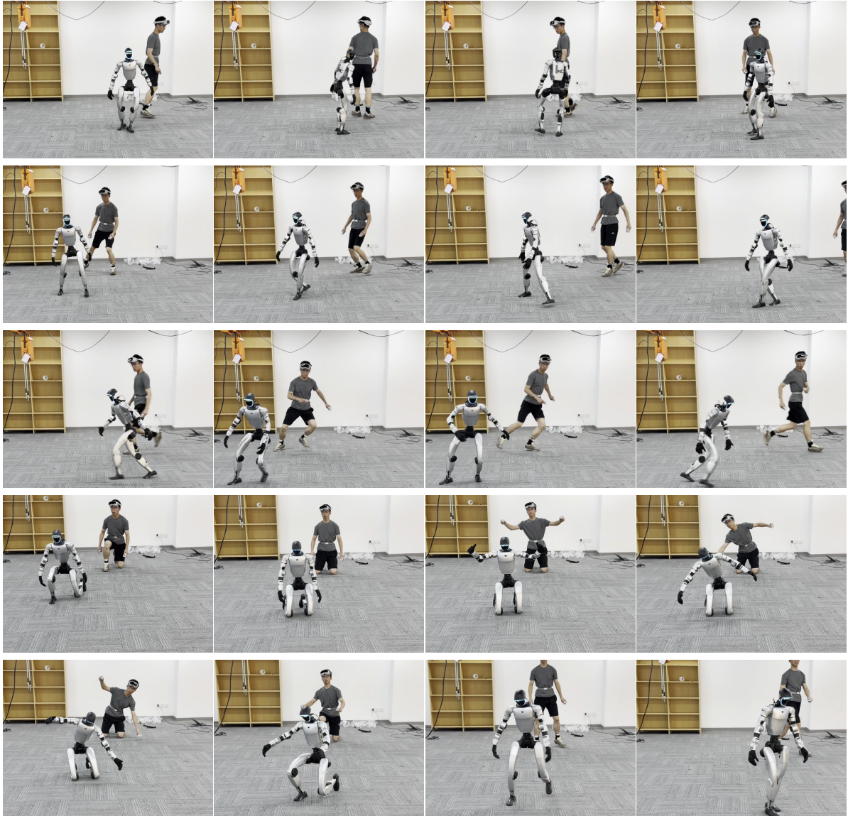
Figure 5: Representative frames from real-robot teleoperation. Rows show turning, side stepping, shuttle running, kneeling down, and standing up; columns show four moments within each motion.
