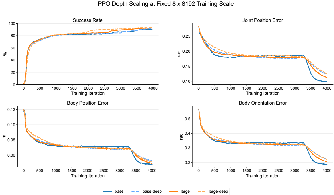
Figure 13: Training curves for depth scaling. Deeper actors can show worse reward-side tracking curves.
