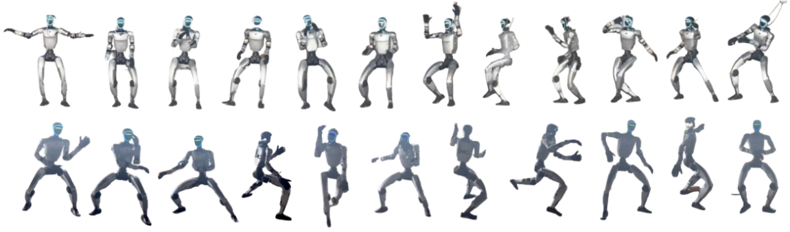
Fig. 6. TeCH performs robust motion tracking on high-dynamic motions in real robot tests.
